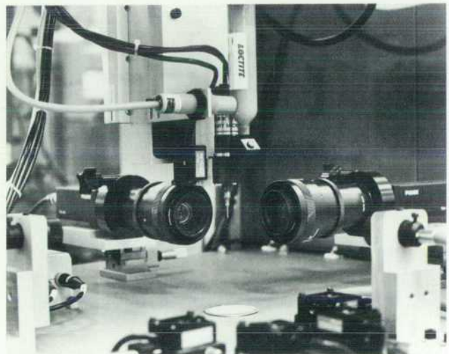
Fig. 2. The adhesive and encapsulant dispensing stations are equipped with two orthogonally positioned cameras using back-lighting to determine the position of the dispensing needle tip accurately.
